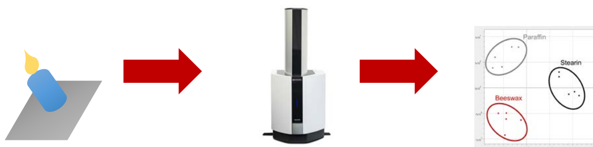
Fig. 1 Workflow: Stuck wax directly from candle → Analyze in MALDI mass spectrometer → Match in statistical software
