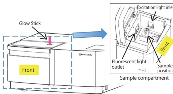
Fig. 4 Diagram of RF-6000 Spectrofluorophotometer and Sample Compartment
